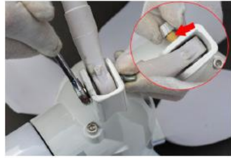
3. Re member to insert the copper tube before assembling the tail
