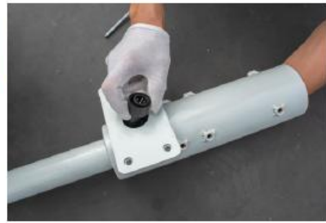
6. Take the wind turbine cables out through the round hole
