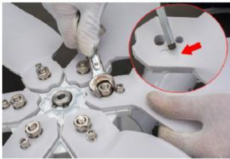
1. Let the blade cover with "Number Mark" face down, and fix it on blade plate with screws
