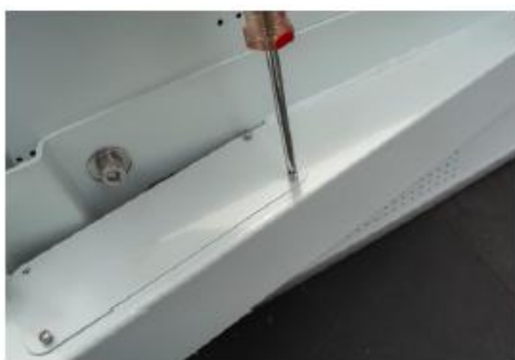
11. Put the connected parts in and lock up the window plate
