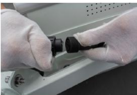
10. Open the window plate, connect the cables and connector
