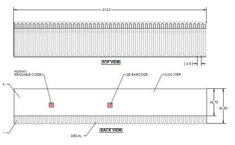
Thin-film CIGS solar cells on stainless steel substrate have high efficiency levels and provide significant advantages over conventional, rigid solar cells.
