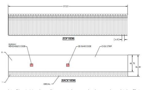
Thin-film CIGS solar cells on stainless steel substrate have high efficiency levels and provide significant advantages over conventional, rigid solar cells.
