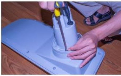
2. Put the Horizontal Bracket on the light body and fasten the screws.
