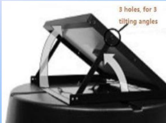
Install the provided screws and brackets left from package to the unit. Then setup the solar panel direction and angle by rotating the regulating plate and adjustment brackets. The optimal adjustment is to have your solar panel 90° to the midday path of the sun.
